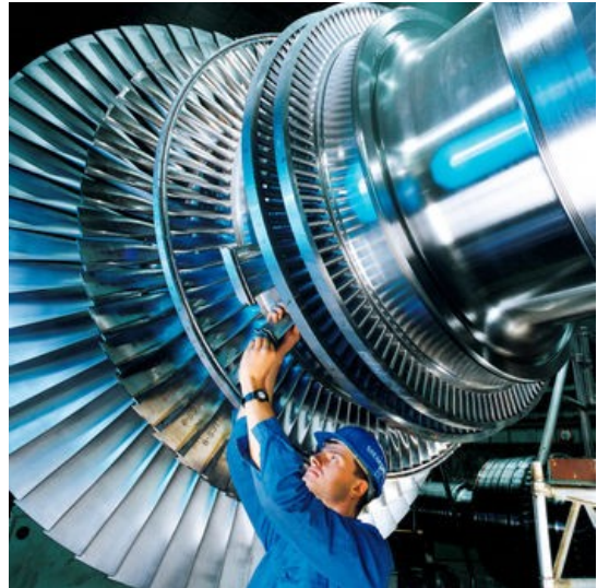
Pic. Turbine rotors on which high-pressure steam is directed
